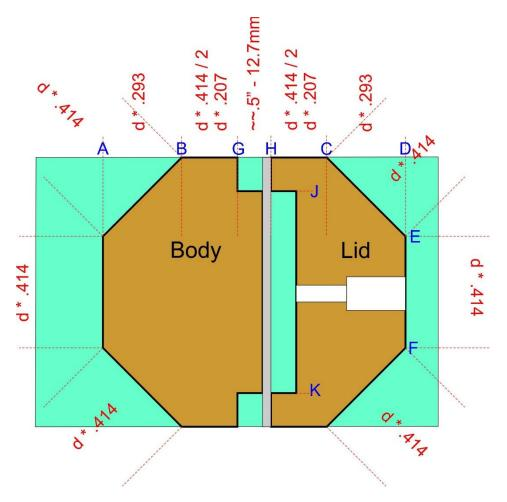
To stretch the octagon, let's add points G and H between points B and C. Line BG is one-half of a side or diameter times 0.207. Line HC is also this same length. The amount of wood is denoted by the line between G and H. It must be enough for the saw kerf and the length of the tenon or depth of the mortise.
