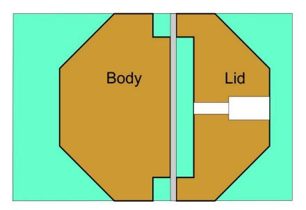
But, hold off from marking these points on the cylinder – We need to create an allowance for the joint. We need to stretch the layout at the joint and allow for enough wood for the parting kerf and wood for the mortise and tenon.
