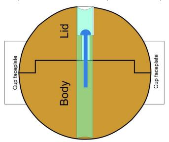
Mount between the cup faceplates. Using two opposite dividing lines and the top screw hole, align the sphere. Use a pencil or other pointing object to follow the line to ensure alignment.
