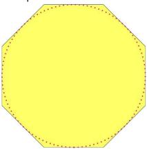
How will an octagon help us? An octagon gives us eight points and eight sides that guide our initial turning. However, since an octagon is a regular polygon, we need only two measures: The length of the octagon's side and the horizontal distance between the right side of the octagon and its nearest corner. More on that later.
