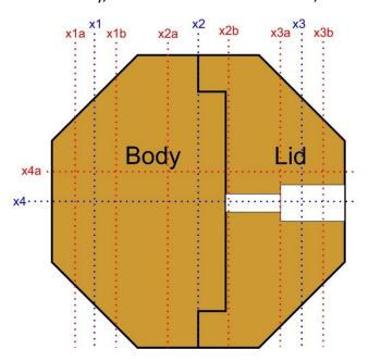
Continue by splitting each surface in half again: Marks x1a, x1b, x2a, x3b, and x4a. Mark both ends of x4a(right and left sides of the octagon.
