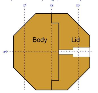
To facilitate rounding off the octagon to become a rough sphere, mark pencil lines at x1 and x3. Each is half of the corresponding side. If the joint is at x2, no additional mark is needed. Theoretically, we should mark x4. However, this is the turning axis and not accessible.
