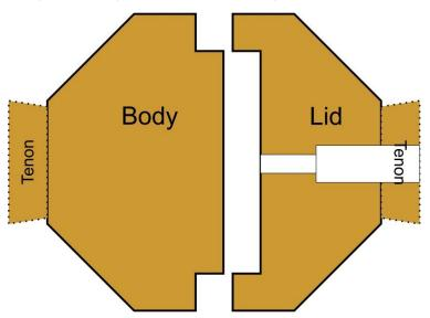
With all points marked on the cylinder and lines drawn around the cylinder by rotating the cylinder under the pencil, we can start serious turning for the exterior of the base and lid pieces. Start by forming tenons on both ends of the cylinder that will securely mount each piece. Then part the two pieces into two individual pieces: Lid and base.
