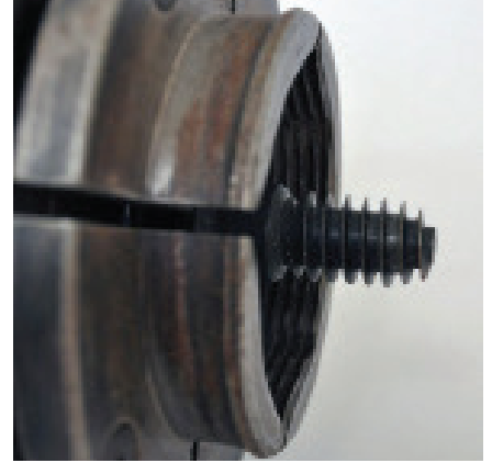
Scroll chuck with woodworm screw
