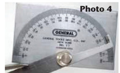
4. Measure the grinding angle of the skew across both bevels. This slender skew has an included angle of 26°.
