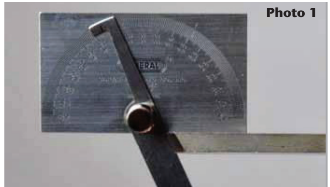
1. Plant the base of the protractor on top of the tool and move the arm to touch the ground bevel. Read the angle, this heavy scraper is 70°, at the mark on the arm.
