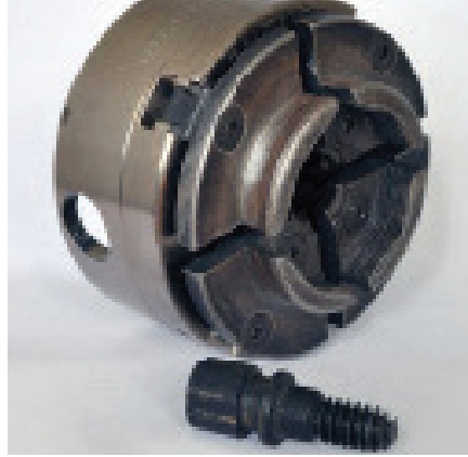
Scroll chuck with woodworm screw
