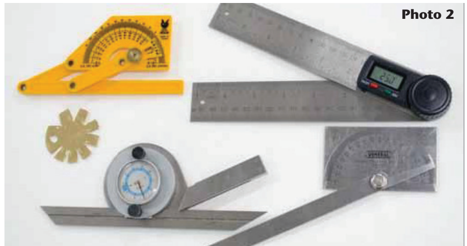
2. Measure the grinding angle with any of these protractors. The round gauge at left is made for turning tools. The simple mechanic's protractor at the right is all you need.
