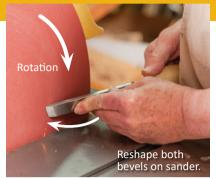
Using the factory-established bevel as a guide, rest one hand on the sander's table, and then swing the tip against the disc or belt, as shown. As you do this, be mindful not to catch the tool's top corner. To avoid a catch, let the skew's bottom edge touch the abrasive before fully registering the bevel against the disc. Repeat this procedure on the opposite face. After grinding both faces, check the bevels, and then make any necessary adjustments so that both bevels are the same length.
