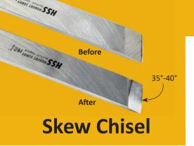
The skew chisel is my go-to tool for most spindle turning. It can be used not only to shape, but also to finish cylinders, V-grooves, beads, and long concave curves. Although it's regarded as the most difficult tool to use, once mastered, it can produce finished surfaces as smooth as the finest grit sandpaper, in a fraction of the time.
