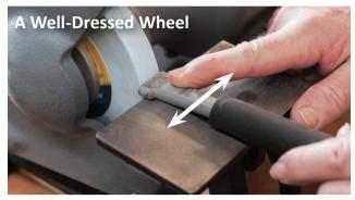
With the rest horizontal at the height of the wheel axis, touch the tool against the wheel and slide it sideways to flatten and clean the surface.
