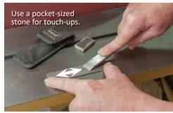
pocket. This accessory provides a handy way to touch up an edge before making a finishing cut. I find that I can re-hone an edge several times before needing to regrind it.
