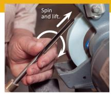
bevel touches the wheel. As you rotate the tool, simultaneously push it up on the grinding wheel, as shown. Repeat this process on one side until sparks come over the edge and inside the flute. Then repeat the procedure on the other side of the bevel. As a final step, rotate outward in both directions from the middle of the gouge's cutting edges to make a uniform, continuous bevel.
