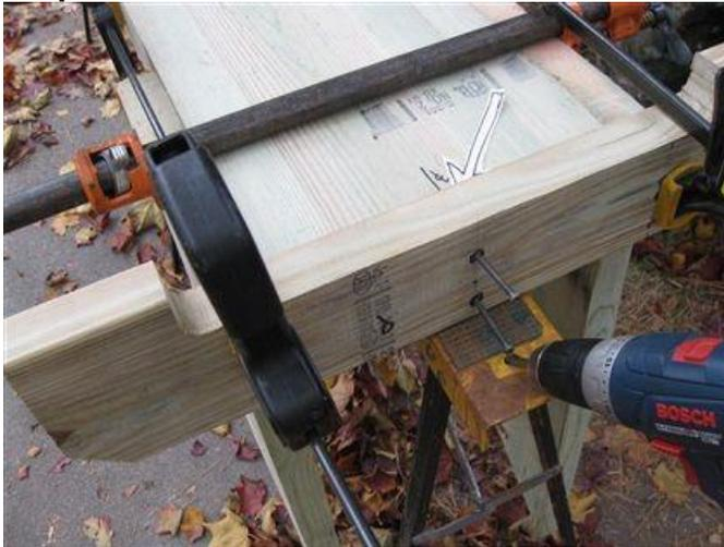
foot and help prevent splitting. (One screw for each of the four points where the feet touch the ground.)
