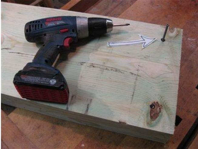
On a flat surface, table or workbench, place the two 2"x12"x27" baseboards on top of the other with the board that has the premarked holes on top. This board will be the bottom baseboard. Screw the two baseboards together with four 2 1/2" screws.
