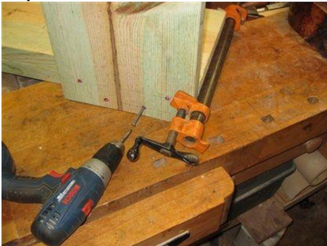
Now with the two baseboards screwed together, Lay on a flat surface, clamp one 45 deg. angled sideboard with its right-side edge flush with the baseboard's end edge. Attach with four 2 1/2" screws.
