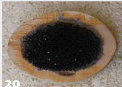
19 With the entire stand held level in a container of uncooked rice, partially fill the hollowed base with resin. Then add weight (in this case, reclaimed shot) and pour more resin until the cavity is filled to the rim.
