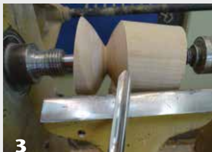
3 With the blank mounted off center, form the first of the V-cuts starting at the headstock end.
