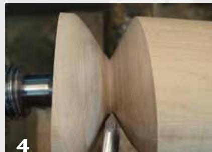
3 With the blank mounted off center, form the first of the V-cuts starting at the headstock end.
