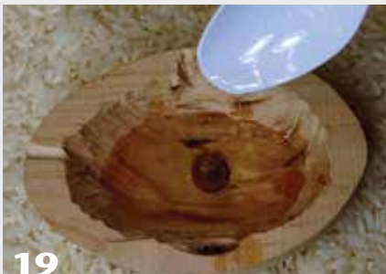
19 With the entire stand held level in a container of uncooked rice, partially fill the hollowed base with resin. Then add weight (in this case, reclaimed shot) and pour more resin until the cavity is filled to the rim.
