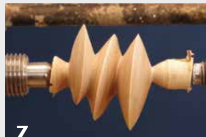
Reposition the blank to a second set of axes and form another V-cut. Repeat this process a third time and complete the turning at both ends, leaving stubs that will be removed later.
