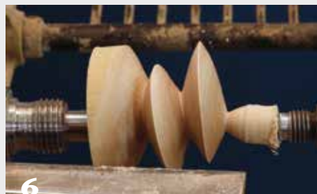
Reposition the blank to a second set of axes and form another V-cut. Repeat this process a third time and complete the turning at both ends, leaving stubs that will be removed later.
