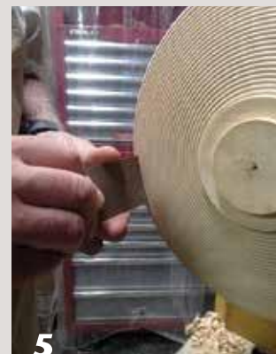
Either stiff sandpaper or a thinned piece of Formica® provides the friction needed to add burn lines in the grooves between beads.
