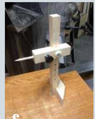
Two versions of pencil-holding jigs. At left, a simpler version, and at right, a more deluxe version allowing easy adjustment of pencil height for use on different-sized lathes.
