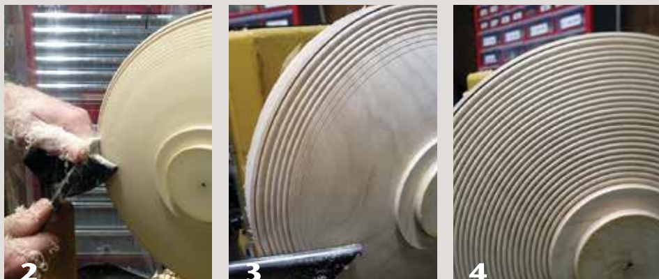
Starting on the bottom of the platter, score and then form beads in one section at a time. With the tool handle down, gently rock the cutting edge left and right until a rounded bead is formed.
