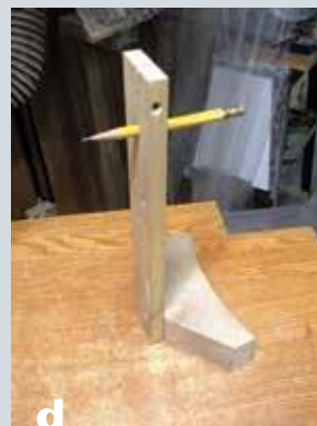
Two versions of pencil-holding jigs. At left, a simpler version, and at right, a more deluxe version allowing easy adjustment of pencil height for use on different-sized lathes.
