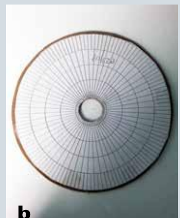
Graph Paper Maker screenshot shows the settings for printing an indexing wheel with 60 and 120 spokes. The printed polar graph is then taped to a hardboard disk and a hole cut out of the center for a completed indexing wheel.
