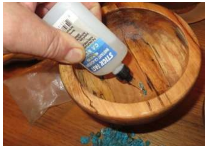
Filling cracks and channels with crushed stone
