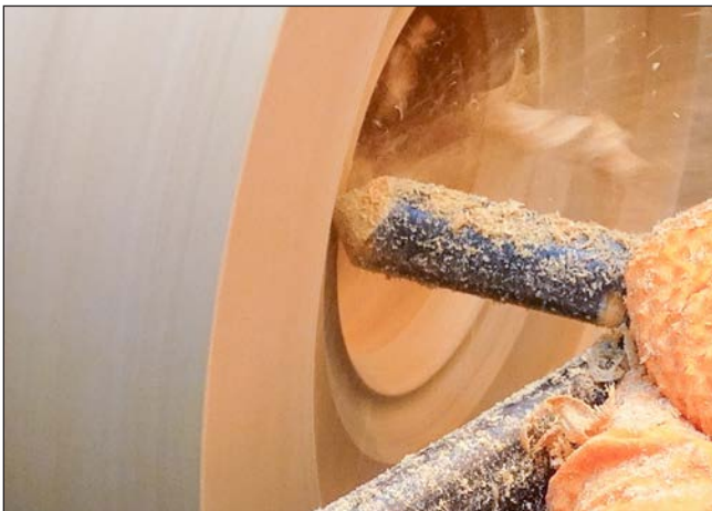
11. Use light shearing cuts to form a transition between the flat recess and the depth hole. This provides clearance for the curve of the stainless-steel screen.
