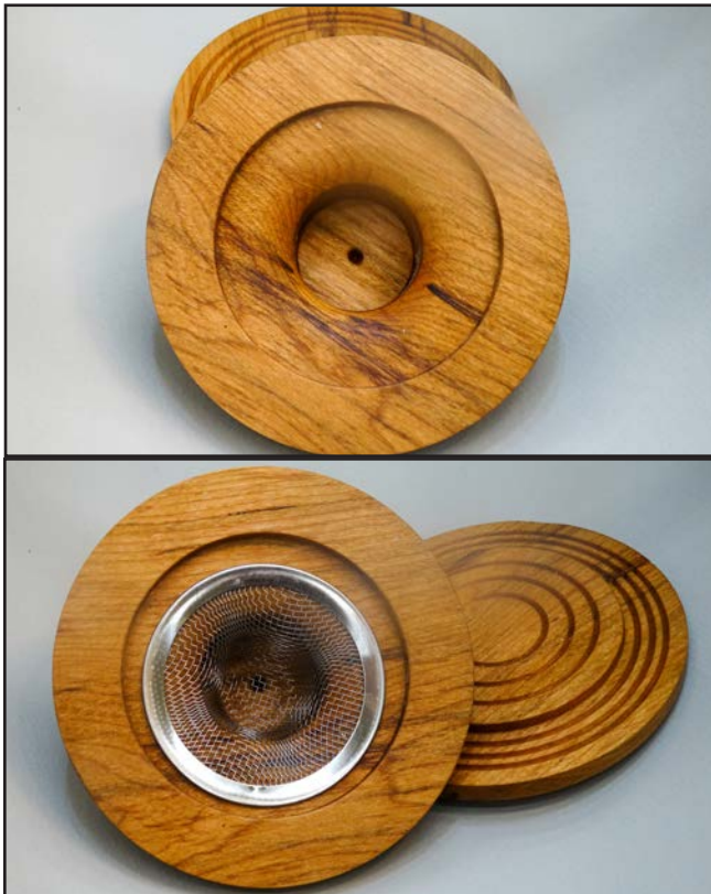
The smoker with and without the essential screen. With the screen removed, note the convex transition into the bottom recess, with a profile that accommodates the curvature of the screen.
