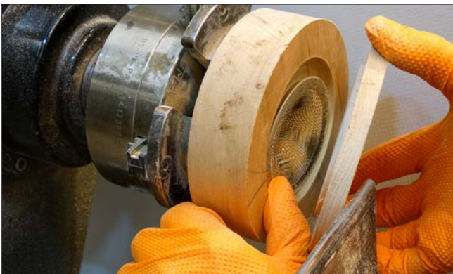
12. Check the fit of the screen and the lid, removing any material that is interfering. You may also want to make the rim around the base's recess slightly concave.
