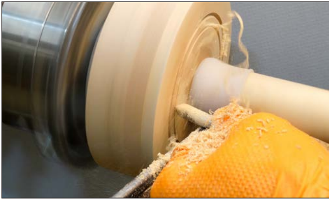
14. Decorate the top of the lid. The author uses a three-point tool to cut grooves.
