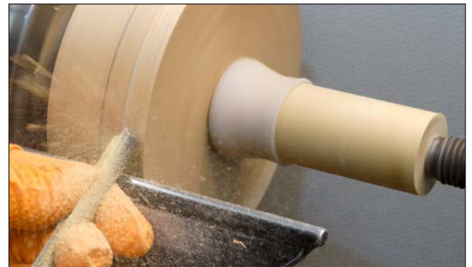
13. Tape the lid to the base and, using tailstock support, true the combined outer rims.
