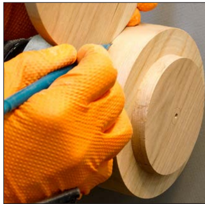
14. Decorate the top of the lid. The author uses a three-point tool to cut grooves.
