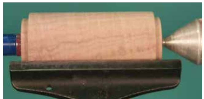
Box blank between centers with tenons on both ends
