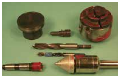
The chuck, drill bits, steb center, screw, and bearing center
