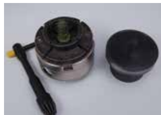
Oneway Talon chuck on left with screw. Screw chuck style faceplate on right.
