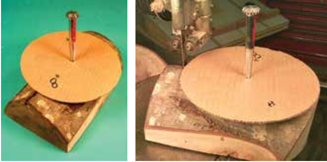
Cutting bowl blank to a circle using a bandsaw
