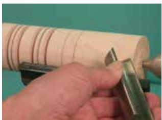
Position of spindle roughing gouge for the planing cut
