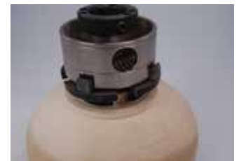
Blank with tenon and square shoulder for mounting in chuck in compression mode
