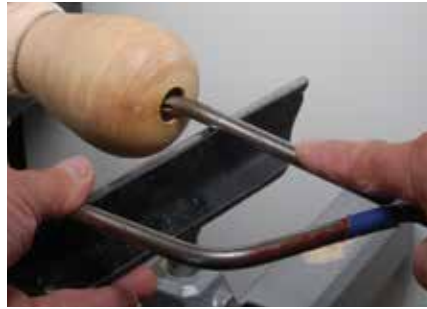
Hollowing tool with outrigger arm
