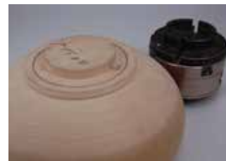
Blank with tenon and square shoulder for mounting in chuck in compression mode
