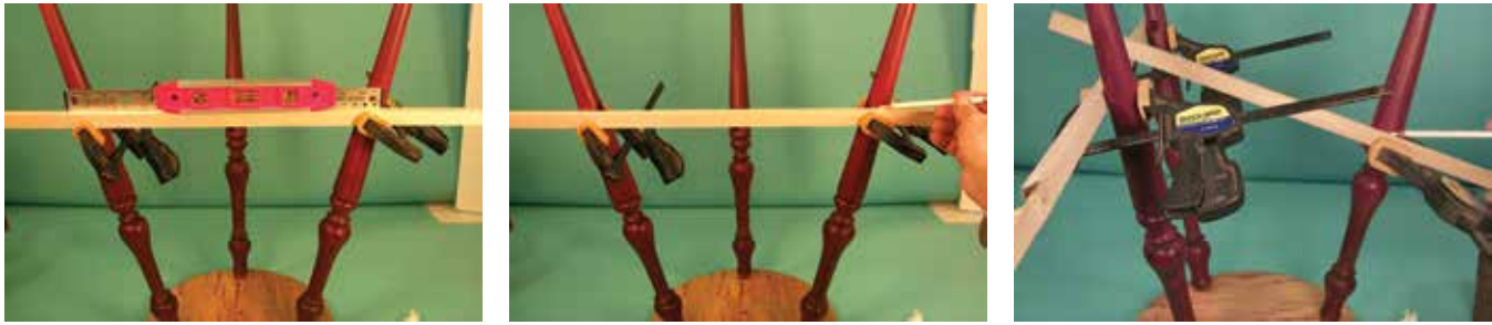
How I mark the angles for the cross braces
