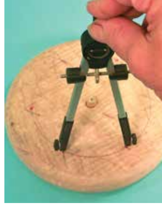
How I lay out and space the holes for the legs, using the radius of the circle to divide the circle with six arcs and then skipping every other arc, mark them for drilling the leg holes
