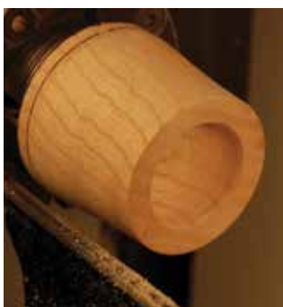
Hollowing cut with spindle gouge
