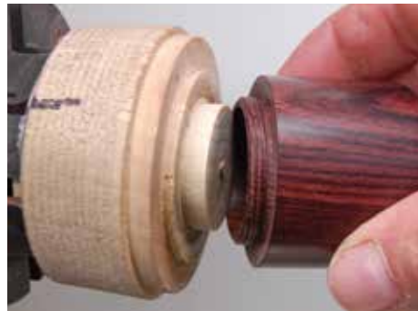
Jam chuck mounted in lathe
