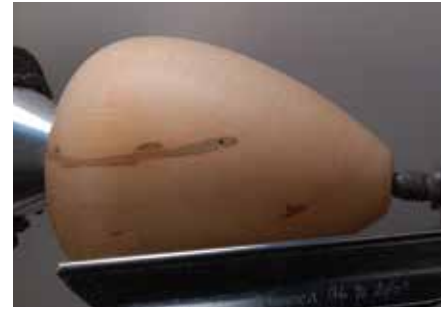
Reverse turning bottom of hollow form
