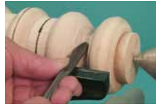
Bottom of cove cut or finished position
