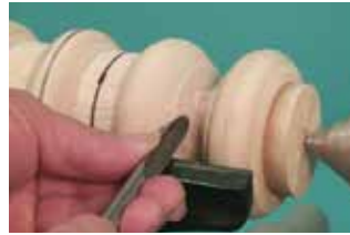
Top of cove cut
