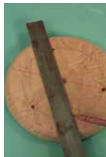
Drawing sight lines for drilling holes. These lines aid in keeping the splay of the legs correct.
