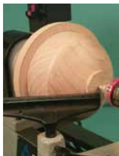
MDF mounted in a four-jaw chuck or on a faceplate with grooves for jam chucking bowl rims for reverse turning
