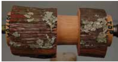
Roughed-turned mushroom mounted in chuck with tenons on both ends
