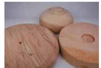
Left front blank with hole drilled for screw chucking. Top has a tenon for compression chucking. Bottom right has a mortise drilled in it for expansion chucking.
