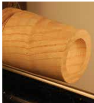
Hollowing cut with ⅜" spindle gouge
