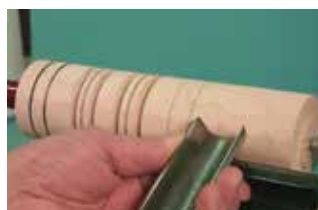
Position of roughing gouge cut
