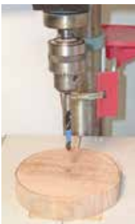
Drilling hole in seat for mounting in screw chuck
