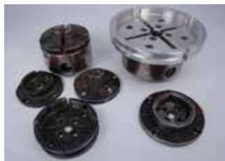
Talon chuck on left, with a variety of jaws. Stronghold chuck on right with #4 jaws.
