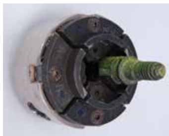
Dimples in side of screw must line up with the tips of the jaws as screw is inserted into the opening between the jaws
