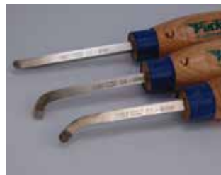
Set of three ¼" Square Packard hollowing tools that have been ground down a bit to minimize torque
