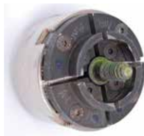
The screw properly inserted into the chuck
