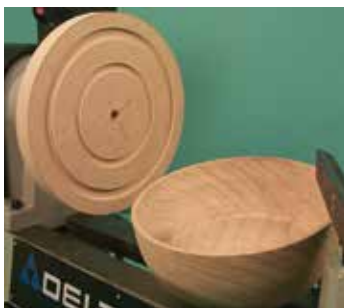
MDF mounted in a four-jaw chuck or on a faceplate with grooves for jam chucking bowl rims for reverse turning
