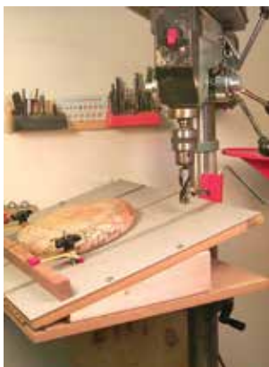
Adjustable drill press table for drilling holes in the seat
