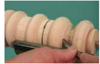
Turning a fillet with flute closed and only the tip cutting
