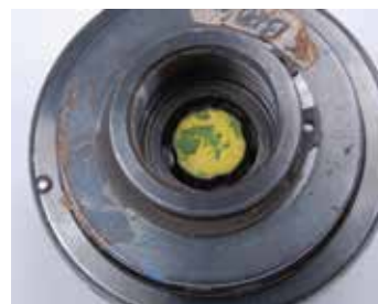
View of screw properly inserted in chuck from the back side of the chuck showing how the tips of the jaws draw in to lock in on the dimples in the screw
