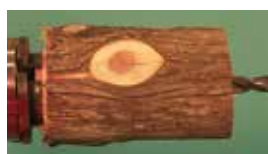
The weed pot mounted between centers after 5/8" hole has been drilled.
