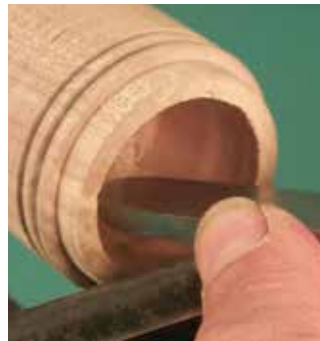
Hollowing inside of box with round-nose scraper
