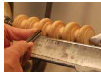
End of bead cut or bottom of bead
