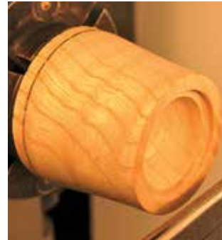
Lid finished and ready for sanding
