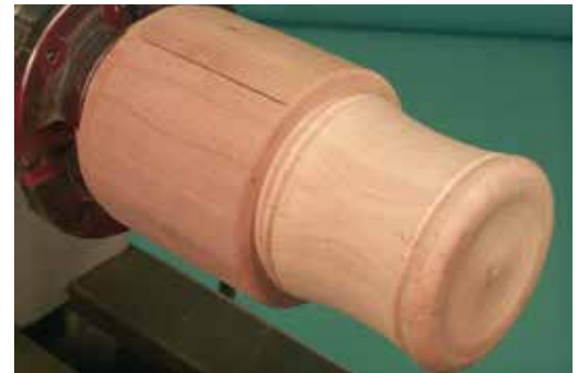
Bottom of box mounted in jam chuck
