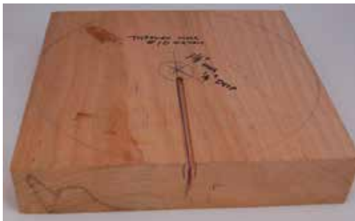
Lamp base with dovetail groove routed in bottom
