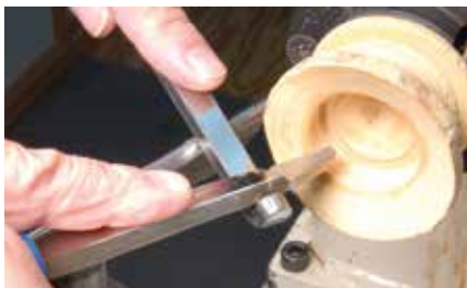
Using thread-chasing arm rest to turn female threads
