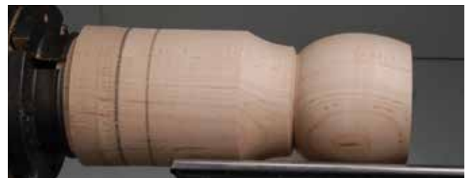
Goblet mounted in chuck with cup partially shaped, ready for hollowing
