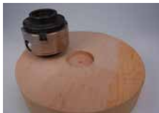
Hole drilled in bottom for expansion chucking
