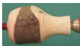
The weed pot mounted between centers after 5/8" hole has been drilled.
