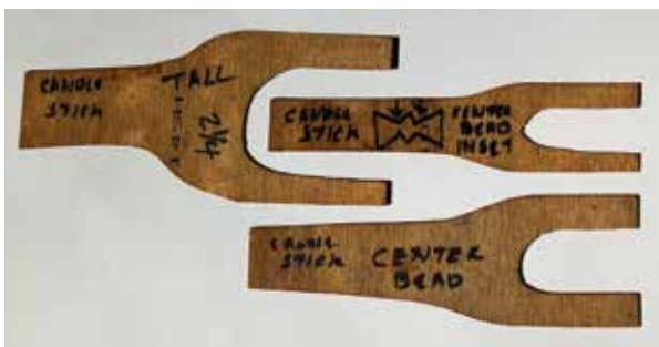
Sample gauges made from Formica
