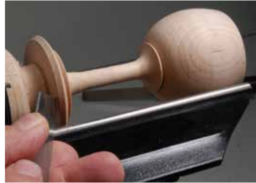
Turning stem with tailstock support
