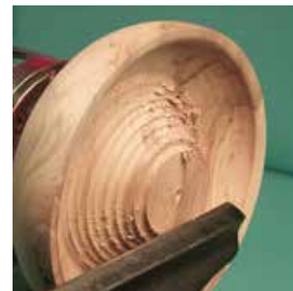
Hollowing a large bowl using the stair-stepping method of leaving material in the center of bowl to minimize flexing of the outside of bowl
