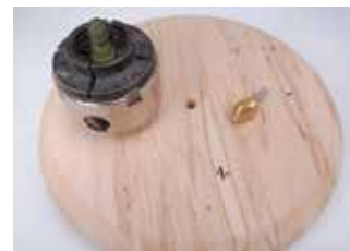
Oneway Talon chuck with screw. Dry blank with \frac{13}{32} " hole drilled in it for Oneway screw and chamfering bit.
