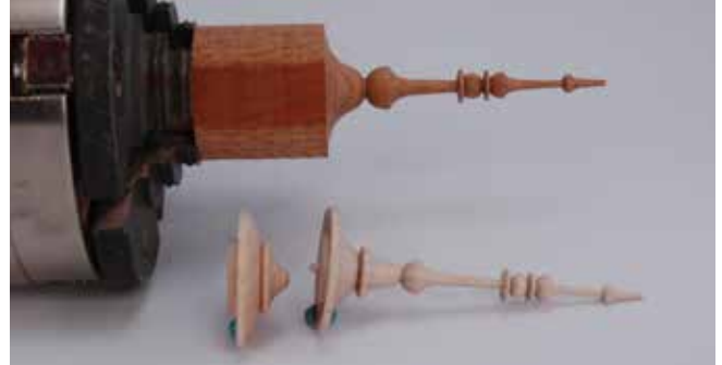
Roughed-out icicle in chuck, turned to a cone shape
