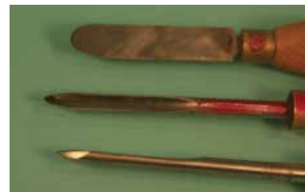
Round-nose scraper (top tool), middle and bottom \frac{3}{8} " spindle gouge top view and side view
