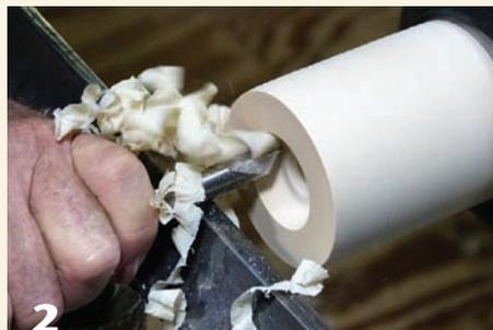
**2** To hollow the inside of the box, cut from the center hole toward the outside edge. I prefer a spindle gouge for this step, but a round-nose scraper will do the job also.
