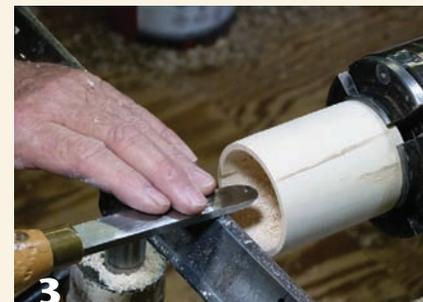
**3** Use a small round-nose scraper to refine the inside of box bottom.
