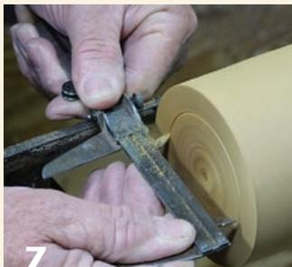
**7** Using calipers, transfer the outside diameter of the box rim to what will become the top of the box.
