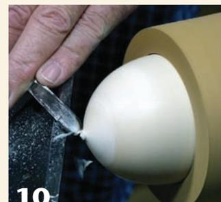
**10** Using the unfinished box top as a jam chuck, finish turning the acorn's bottom.
