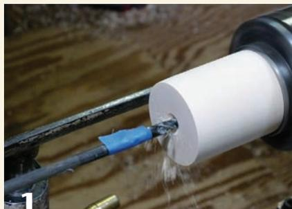
**1** With the blank re-chucked and trued up, drill a center hole to aid in the endgrain hollowing.
