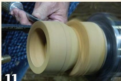
11 Shape the outside of the acorn cap, sand only the inside, and part off.
