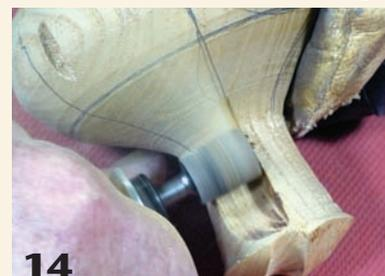
14 With the main carving sections laid out, begin shaping with a burr and rotary tool.
