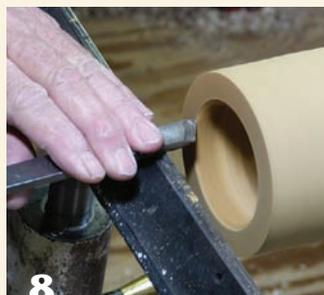
**8** After hollowing the box top, gradually reduce the inside diameter of its rim until the bottom fits inside with a good friction fit.
