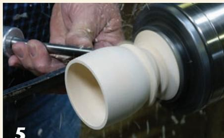
**5** Shape the outside of the box, being careful not to cut through its bottom.
