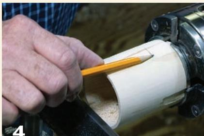
**4** Make a pencil line on the outside of the box indicating the inside depth. This is an important reference for when you begin to final-shape the outside of the box.
